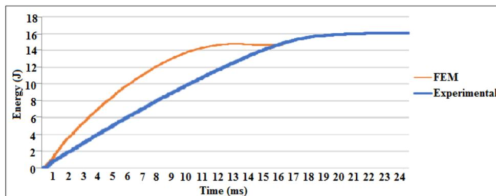
**Figure 14.** The energy absorbed during the impact (PLA 5% 15J)
