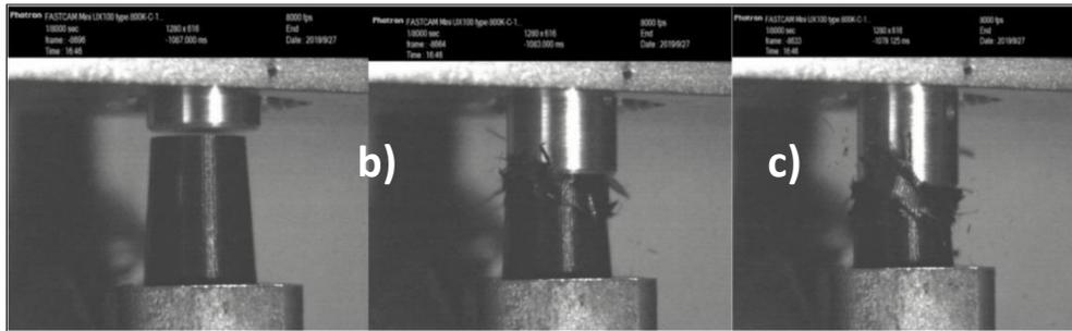
**Figure 10.** 10% honeycomb specimen, impacted at different timeframes: a)  $t=0$  ms, b)  $t=1.3$  ms, c) maximum displacement; 40 J impact loading
