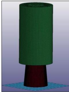
**Figure 5.** Components of the numerically modeled part; fixed rigid plate can be seen on the bottom side (blue), continuing with the honeycomb structured part and the impactor (green)
