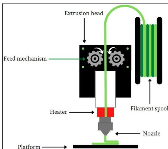
**Figure 1.** FDM process scheme
