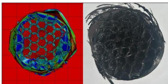
**Figure 16.** Honeycomb buckling (comparison between finite element modeling and tested specimen)
