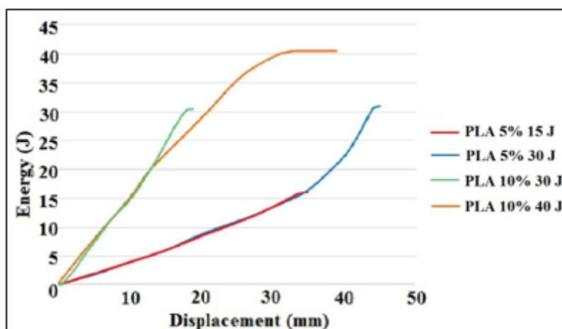
**Figure 7.** Energy (J) - displacement (mm) curves of the tested structures
