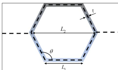
**Figure 3.** Layout of the hexagonal cell
