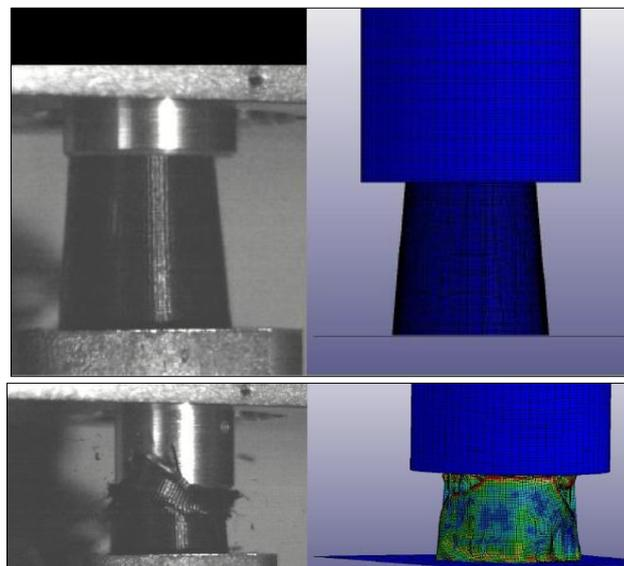
**Figure 11.** Comparison of the maximum displacements between the finite element model and the real model before and after the impact (PLA 5% 15J)
