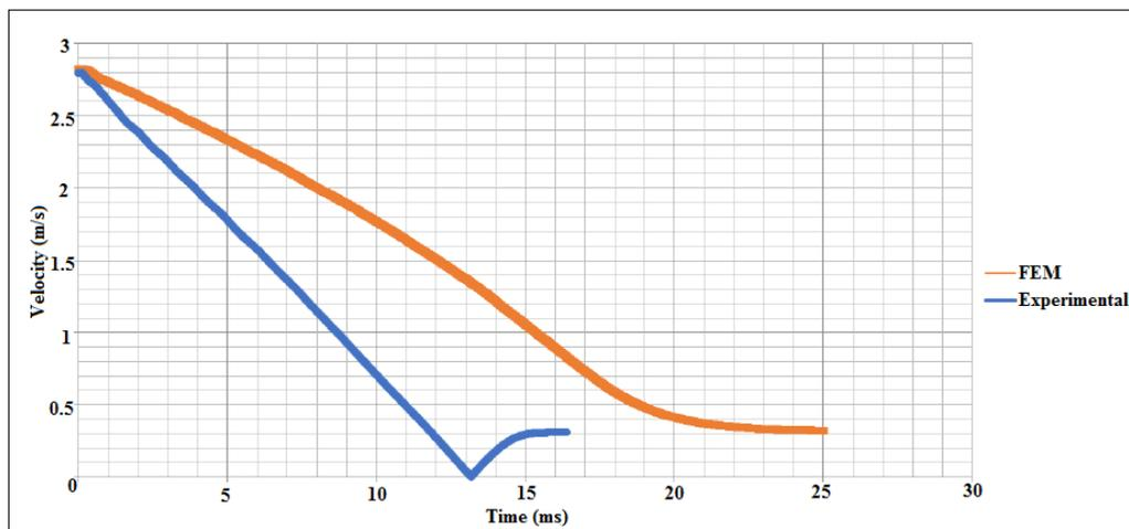
**Figure 15.** Velocity variation in the finite element model and experimental results (PLA 5% 15J)
