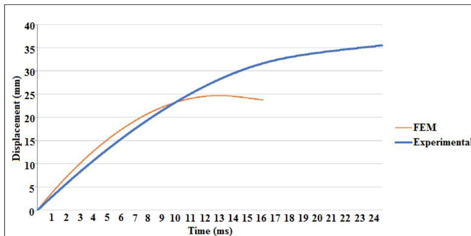
**Figure 13.** Comparison of displacements in the finite element model and experimental results (PLA 5% 15J)
