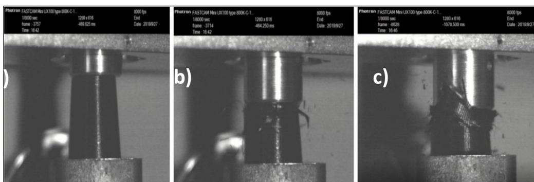
**Figure 9.** 5% honeycomb specimen, impacted at different timeframes:
