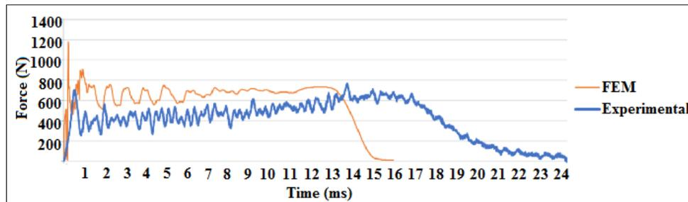
**Figure 12.** The dynamic response of the structure obtained with the finite element method and by processing the experimental data (PLA 5% 15J)
