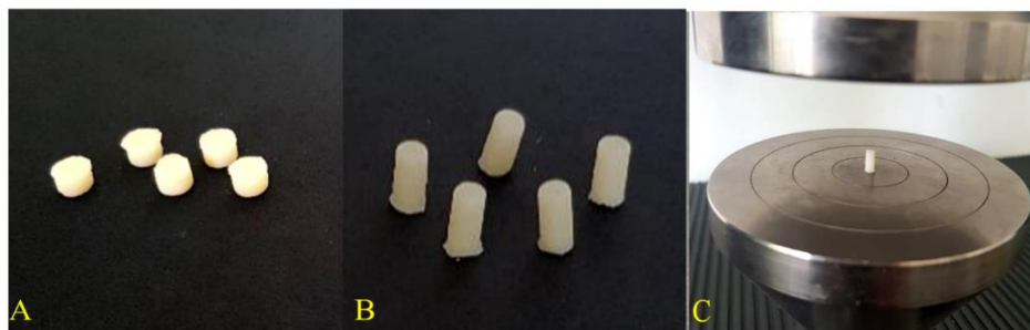
Figure 1. Standard composite samples (A, B); HV testing device (C)
