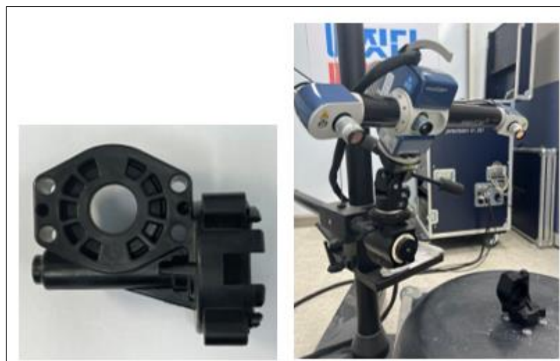
Figure 10. 3D scanning for checking amount of deformation in wheel speed meter housing
