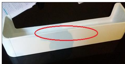
Figure 1. Shows the part under study with the deformation detected at the outlet of the mold and after cooling
