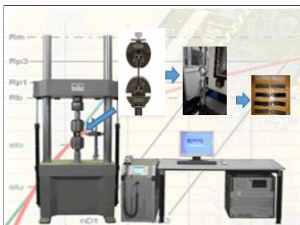
Figure 3. The mechanical testing machine for determining of tensile strength in static regime of materials, with adapted device and samples broken after elongation
