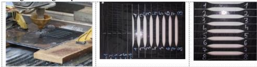
Fig. 2. Water jet cutting 2a (left). The entire material with cut samples 2b (center). The tensile tests samples 2c (right)
