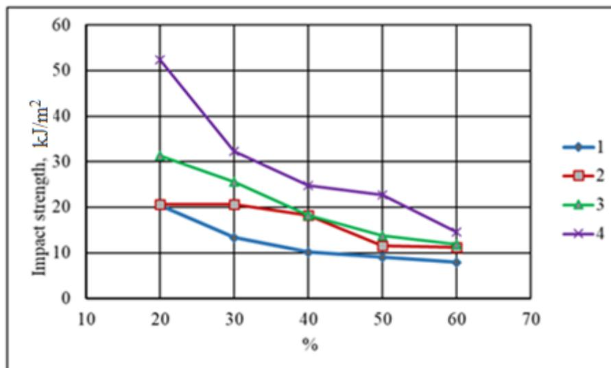
**Figure 5.** The LDPE impact resistance development curve depending on the percentage of organic fillers 1) wood powder, 2) medium-sized wood, 3) long wood, 4) random particles
