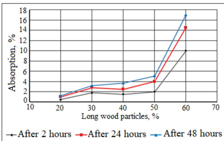
**Figure 10.** The fresh water absorption by RLDPE samples as the percentage of an organic filler - long particles
