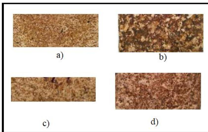
**Figure 3.** an artificial wood sample made from: a) 60% wood powder + 40% RLDPE, b) 20% large particles + 80% RLDPE, c) 50% medium particles + 50% RLDPE, d) 30% long particles + 70% RLDPE
