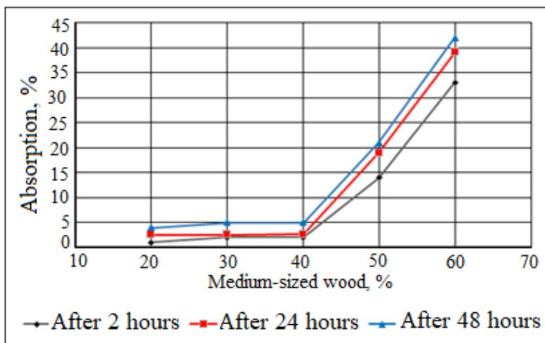
**Figure 8.** The fresh water absorption by RLDPE samples due to the percentage of organic fillers - medium-sized particles
