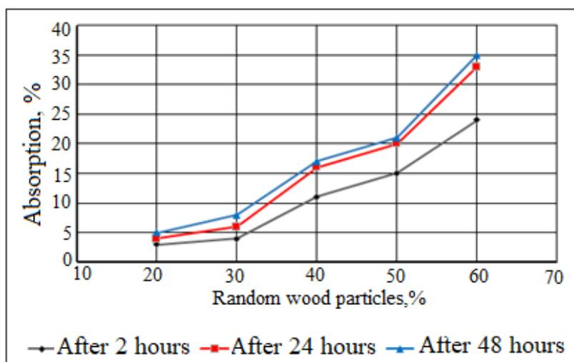
**Figure 12.** Fresh water absorption by RLDPE samples as the percentage of organic fillers – random particles
