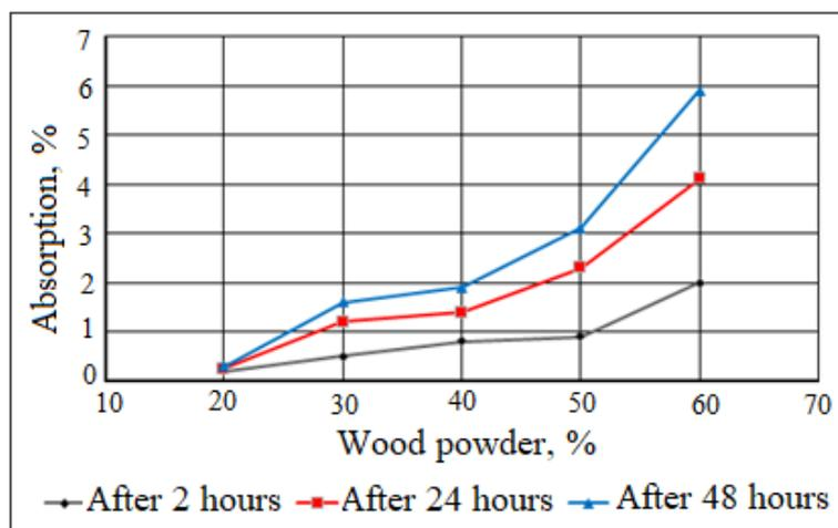
**Figure 7.** The salt water absorption by RLDPE samples depending on the percentage of wood powder
