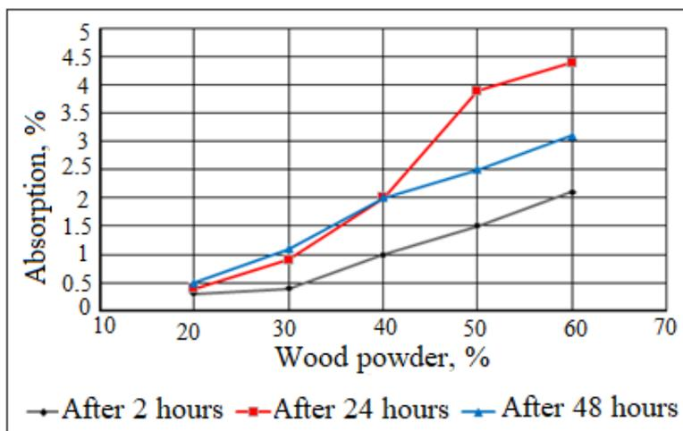
**Figure 6.** The fresh water absorption by RLDPE samples depending on the percentage of wood powder
