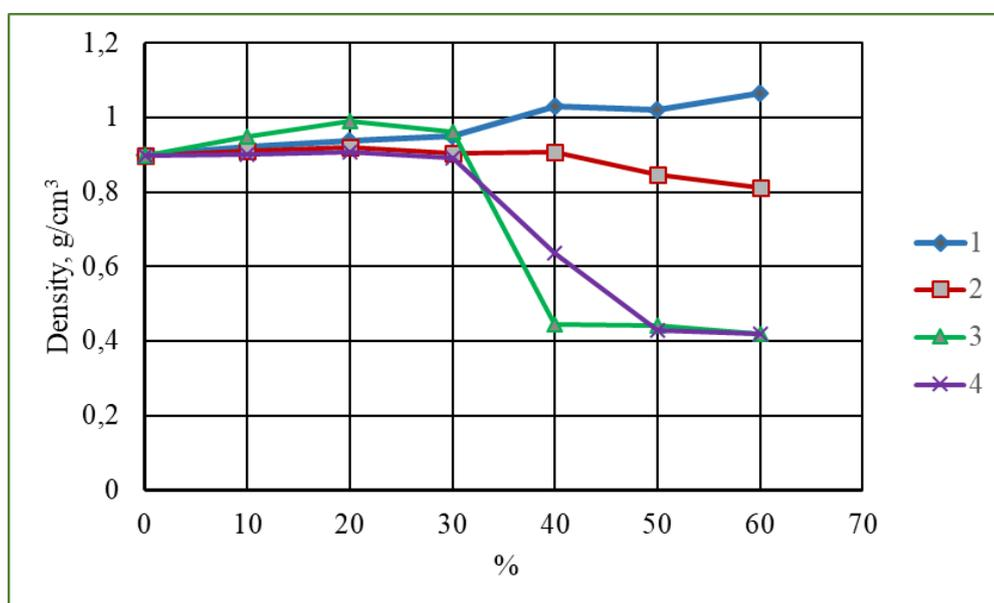
**Figure 4.** The RLDPE composites density development curve containing different proportions of a 1) wood powder, 2) medium-sized wood, 3) long wood, 4) random set of wood particles as an organic filler
