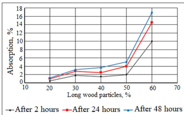
**Figure 11.** The salt water absorption by RLDPE samples as the percentage of an organic filler - long particles
