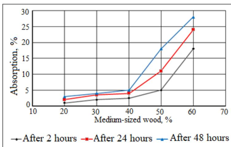
**Figure 9.** The salt water absorption by RLDPE samples depending on the percentage of an organic filler – medium-sized particles
