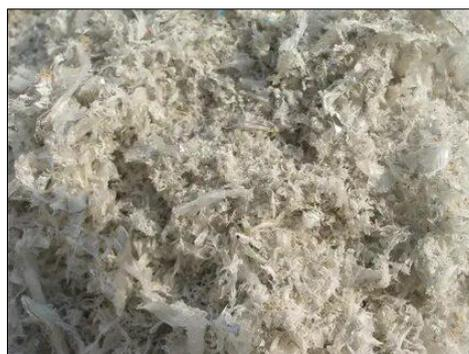
**Figure 1.** Low Density Polyethylene (RLDPE)
