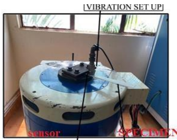
Figure 2. Computerized Free Vibration set-up used in this experiment
