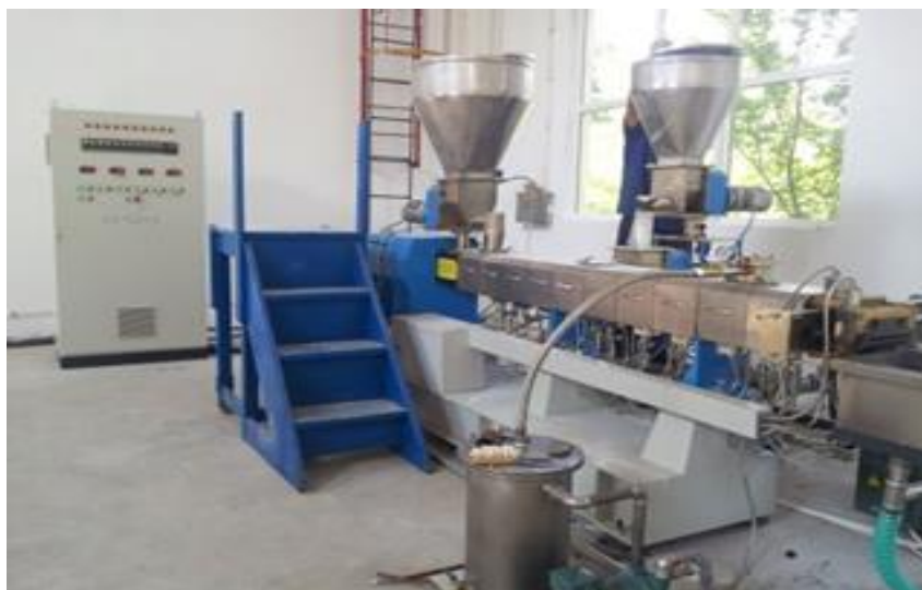
Figure 2. EC 52 double screw granulator extruder (SC Monofil Săvinești SA, Romania)
