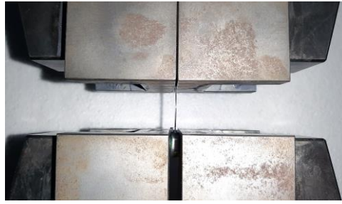
Fig. 6. The setup for the tensile breaking force tests.
