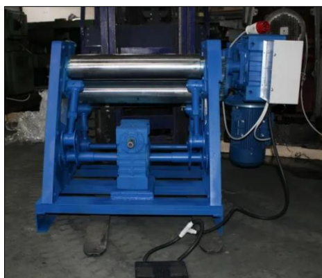
Figure 1. The rolling machine for forming samples
