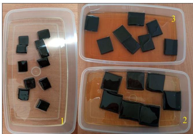
Figure 8. The solvent testing of samples (1- gasoline, 2- diesel fuel, 3- technical oil)
