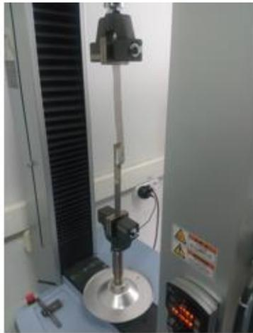
**Figure 1.** Material test for peel strength from metal
