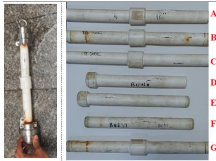
Figure 6. Samples subjected to burst pressure tests
