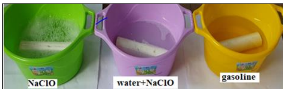
Figure 3. Immersion of PPR pipes in chemically active environments
