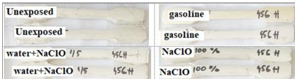
Figure 8. The aspect of the samples used for tensile test
