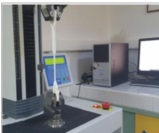
Figure 9. Device used for tensile test of PPR pipes
