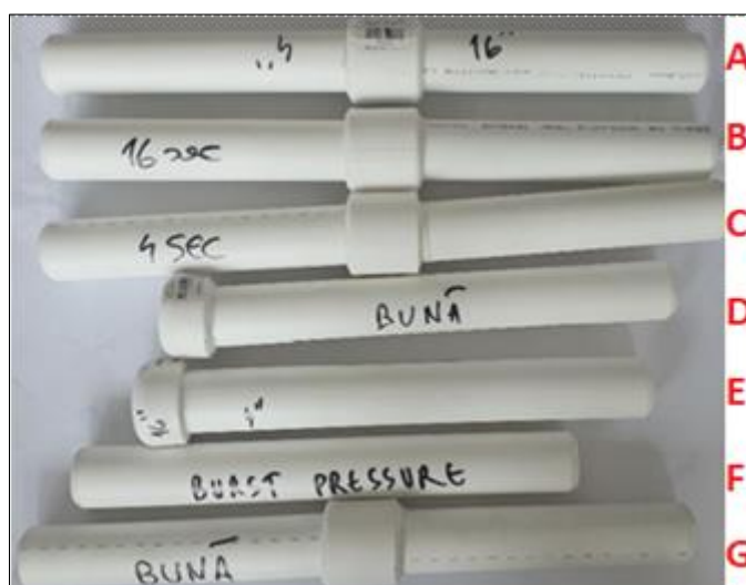
Figure 2. The aspect of the welded PPR pipes
