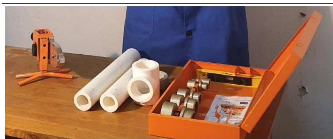
Figure 1. The joining elements used in the experimental investigation
