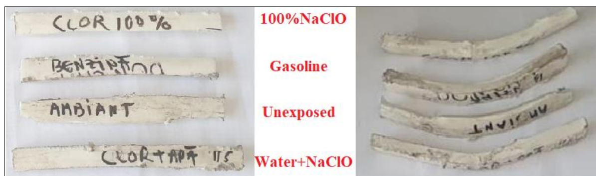
Figure 11. Bending test of PPR pipes before (left) and after (right) the test
