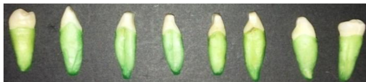
Fig. 5. Roots covering with a 0.3 mm calibrated layer of wax
