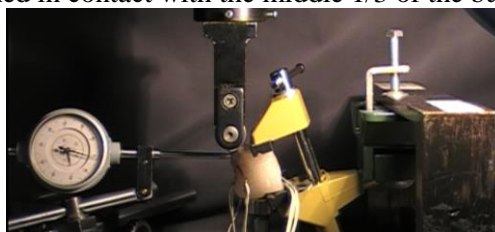
Fig. 10. The probe application on the buccal surface of the lateral incisor
