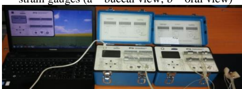
Fig. 8. Strain gauge bridges P3 model (Vishay)
