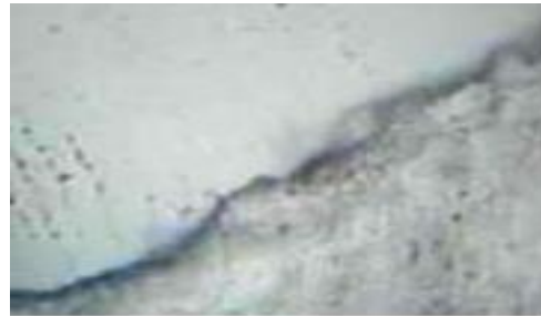
Fig. 9. The interface between the ceramic restoration and the Variolink N resin after the immersion in artificial saliva
