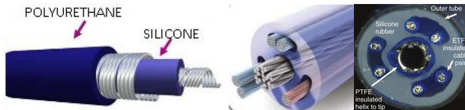
Fig. 2. Bipolar coaxial pacing lead design . ETFE = ethyltetrafluoroethylene; PTFE = polytetrafluoroethylene (from thoracickey and Medtronic)
