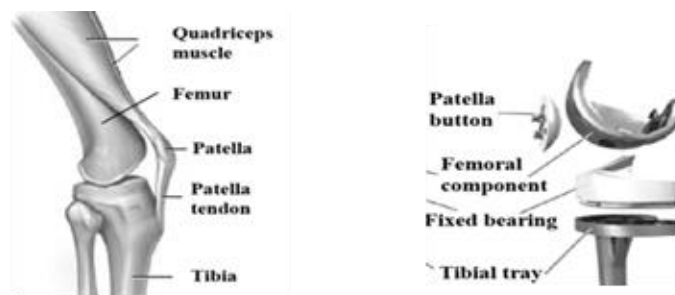
Fig.1 (a)Knee joint anatomy, (b)Knee prosthesis (arthroplasty) (adapted Junfen Shi (2007)) – Finite Element Analysis of total knee replacement considering the gait cycle load and malalignment, PhD Thesis University of Wolverhampton, 2007, https://core.ac.uk/download/pdf/1931943.pdf , pag.6(fig.1(a)), pag 31(fig.1(b))
