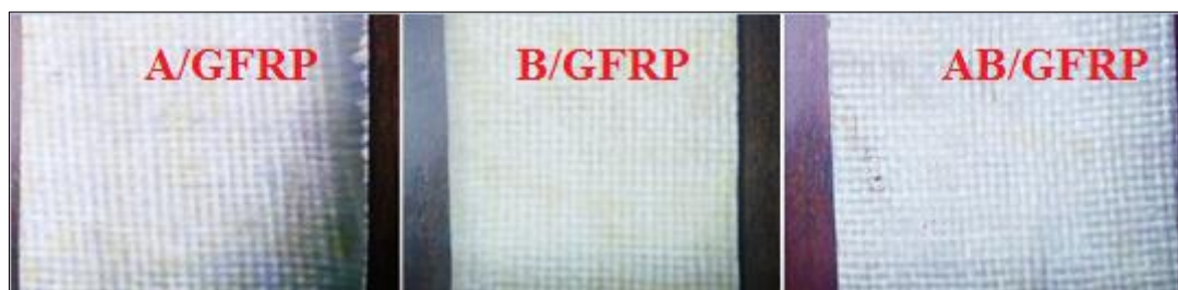
Figure 1. Fabrication sheet of aluminium glass fiber polyester laminate(A/GFRP), Bentonite glass fiber polyester laminate (B/GFRP) and combined aluminium & Bentonite glass fiber polyester laminate (AB/GFRP)
