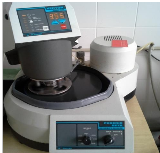
Figure 3. The Buehler VECTOR machine where the samples were polished
