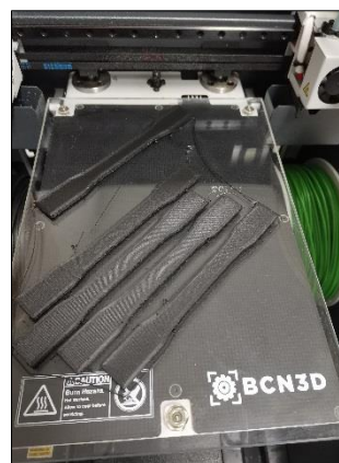
Figure 5. Specimens position on the printing platform
