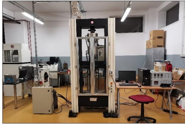
Figure 6. WDW-150S Universal Testing Machine
