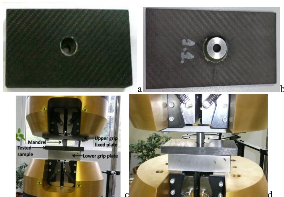
Figure 3 Metallic insertions Design 1 hybrid metallic/composite sample a) upper and b) bottom tested side images; c) during compression „pull-out” testing sample; d) dedicated testing device, mounted on the Instron 8802 testing machine
