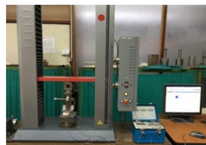
Fig. 3. The strain bridge connected to the computer
