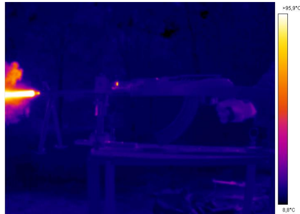
Fig. 2. The hot gases coming out of the barrel behind the projectile
