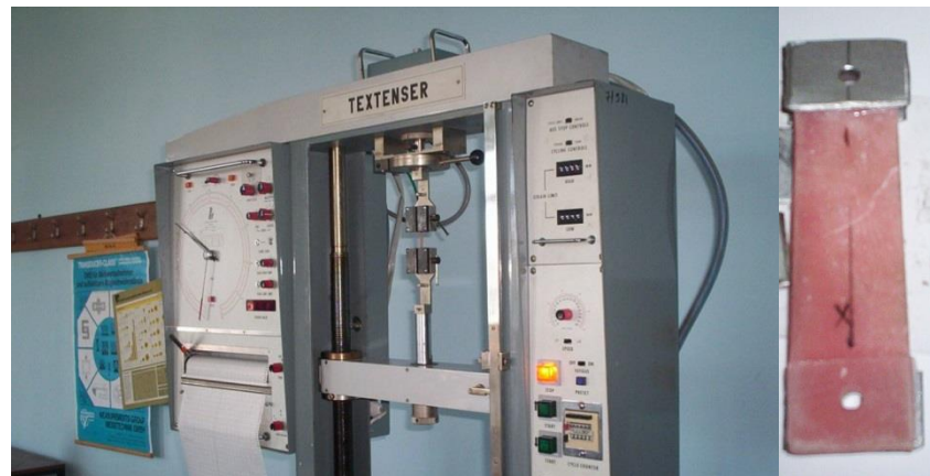
Figure 3. Trial Textener machine and test specimen
