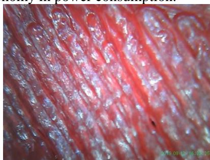
Fig. 8. Deposition shape in lower extrusion temperature
