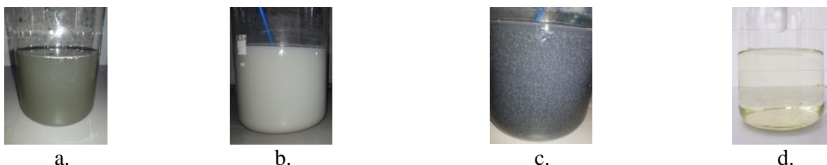
Figure 4. Intermediate stages of the experimental work no. 3 (pH of destruction = 3): (a) Initial wastewater; (b) Addition of \text{H}_2\text{O}_2 ; (c) Addition of \text{FeCl}_3 and \text{H}_2\text{PO}_4 ; (d) Resulted treated water
