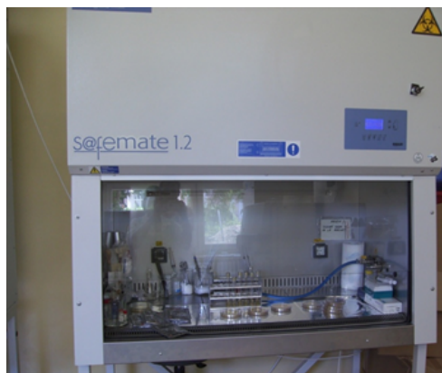
Fig.1. Aseptic enclosure in the class II microbiological hood
