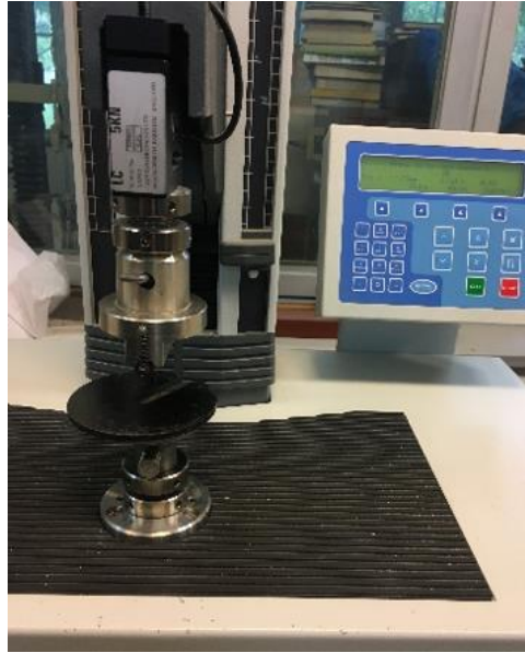
Fig. 1. The universal Loading Machine (Lloyd Instruments)
