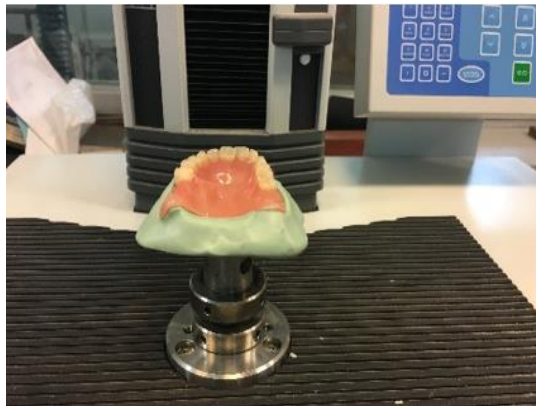
Fig. 2. Fractured specimen from the classical acrylic complete dentures group
