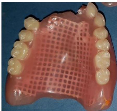
Fig. 8. Metal reinforced acrylic maxillary denture fractured mostly peripheral, outside the metal mesh zone
