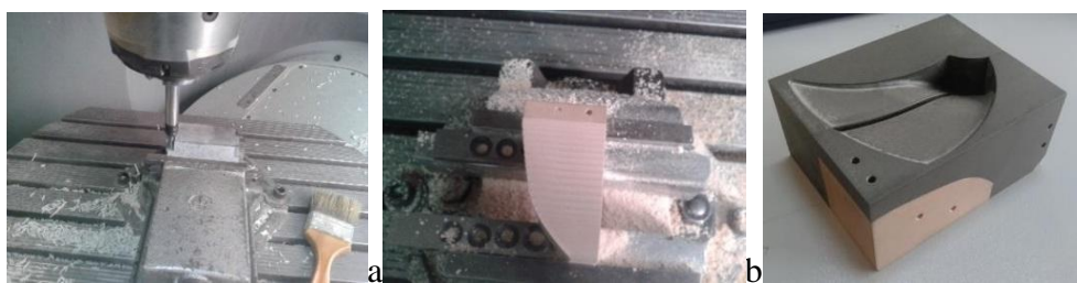
Figure 8. Machining of a) N1001; b) N651; c) final Necuron mould (scale 1:2.5)
