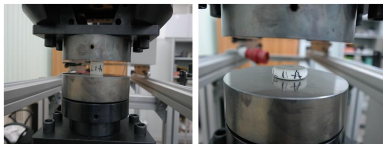
Figure 6. Before and after mechanical stress of specimens
