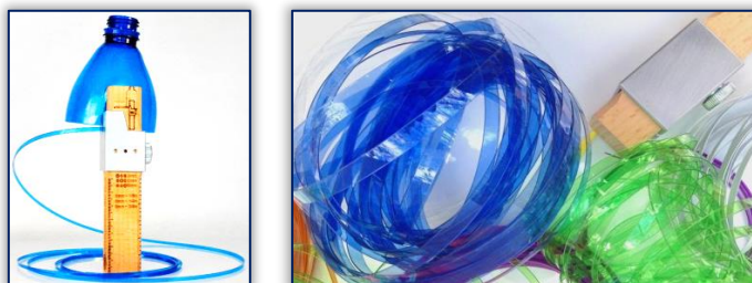
Figure 2. Extraction of long flat strips (yarns) from polyethylene terephthalate (PET)
