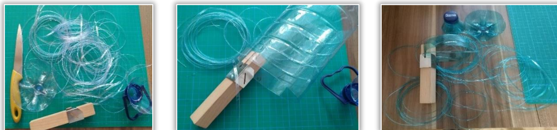
Figure 4. Extraction in yarns and obtaining the long polyethylene terephthalate (PET) yarn
