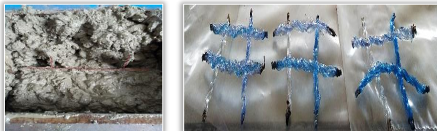
Figure 10. The PET flakes reinforcing process with PET rope strands
