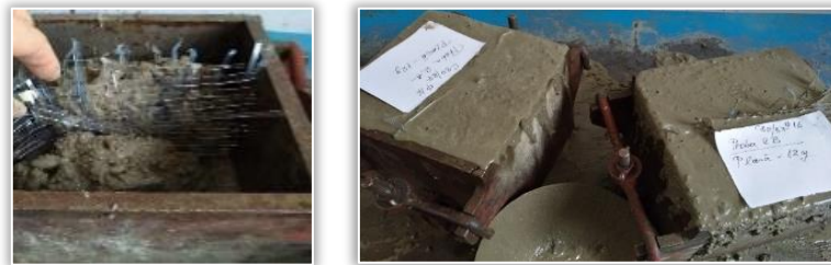
Figure 9. The reinforcing process with PET mesh-shaped woven and labelling the samples
