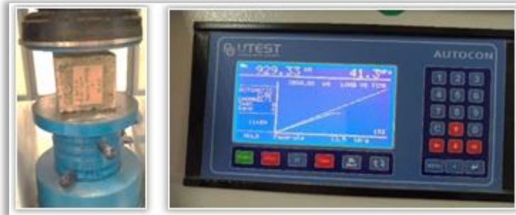
Figure 12. Compression strength test of with PET mesh-shaped woven' reinforced concrete samples
