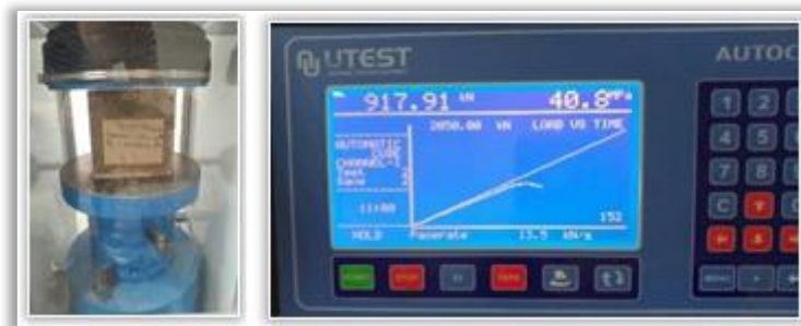
Figure 13. Compression strength test of with PET rope strands' reinforced concrete samples
