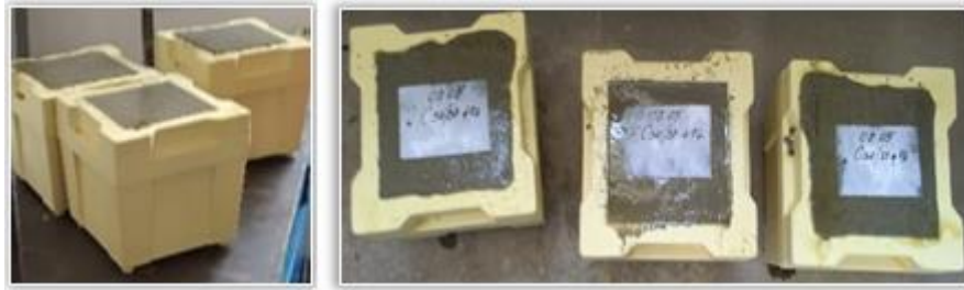
Figure 8. Preparing and labelling the concrete samples
