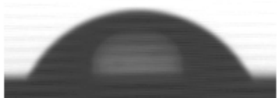
Fig. 1 Image of the water drop deposited on CS2 sample - cement with lowest contact angle
