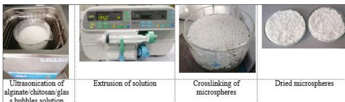
Figure 1. Obtaining of alginate/chitosan/glass bubbles microspheres
