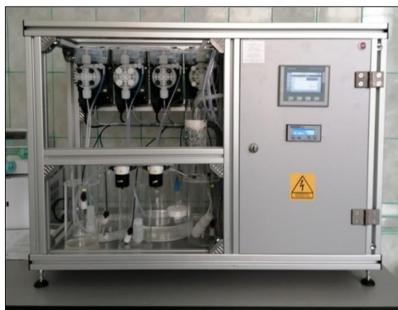
Figure 2. Testing stand for removal of Cu(II) with the alginate/chitosan/glass bubbles microspheres
