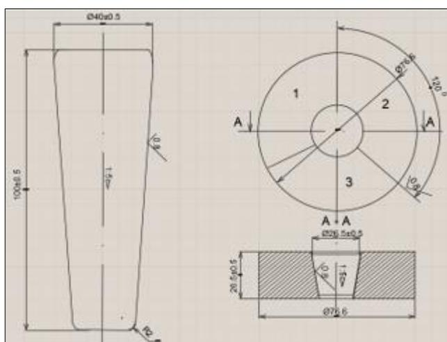
**Figure 4.** Device used in internal pressure test on PEHD ring
