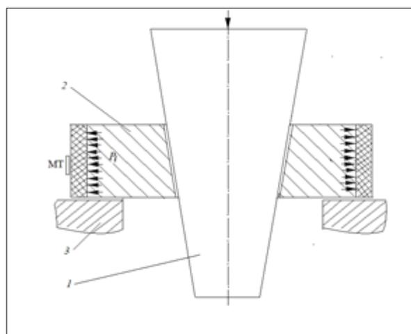
**Figure 5.** Schematic of the internal pressure test of a PE100 pipe ring
