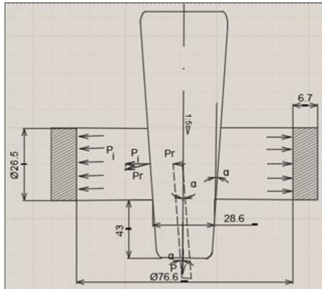
**Figure 8.** The diagram for the analytical calculation of the internal pressure
