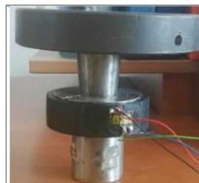
**Figure 7.** The appearance of the tensometric marks on the body under test
