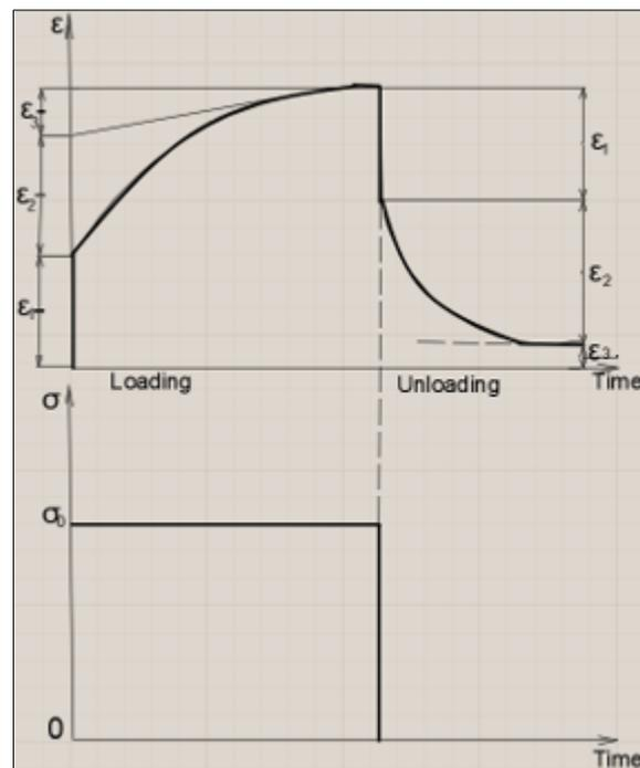
**Figure 1.** The relation between strain and time in a plastic specimen subjected to constant stress  $\sigma_0$
