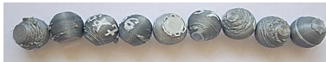
Figure 4. Test pieces obtained by 3D printing before applying the axial compression tests
