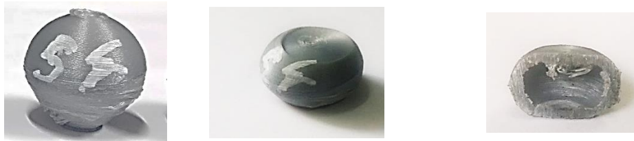
Figure 7. The aspect of the initial part shape, of the deformed part after the application of the compression test and the internal surface that corresponds to the deformed part (initial part thickness h=2 mm, printing speed v=75 mm/s, cooling level c=50 %, plate temperature \theta=65^{\circ}\text{C} )
