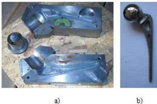
Fig. 1. Tool for meltable implant model a) and finished hip implant metal cast piece b)
