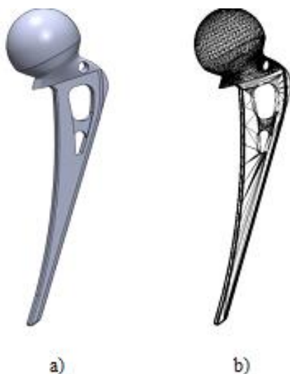
Fig. 3. Visual display of the hip implant model: SolidWorks model a) and STL model (9580 triangles) b) [22]
