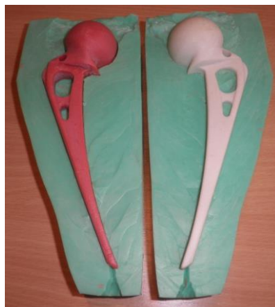
Fig. 7. Silicone rubber mould, wax pattern (left) and 3DP master pattern (right) of hip implant Austin Moore
