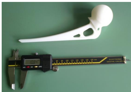
Fig. 8. Digital calliper and ABS pattern of hip implant
