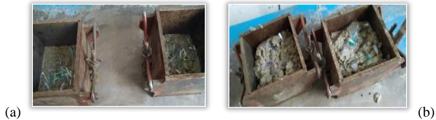
Figure 7. The PET flakes reinforcing process: a) with PET flat strips; b) with PET chips
