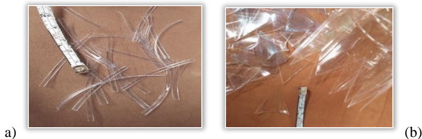
Figure 4. Preparing the PET reinforcement: a) PET flat strips; b) PET chips
