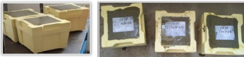
Figure 6. Preparing and labelling the concrete samples
