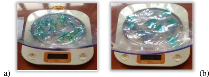
Figure 5. Weighing of the PET flakes reinforcement: a) PET flat strips; b) PET chips
