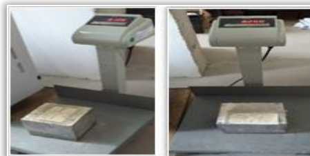
Figure 9. Weighing of the concrete samples
