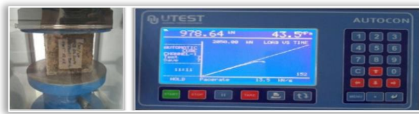
Figure 11. Compression strength test of with PET chips' reinforced concrete samples
