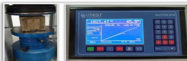
Figure 10. Compression strength test of with PET flat
