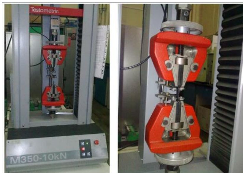
Figure 2. Universal testing machine Testometric M350-10kN
