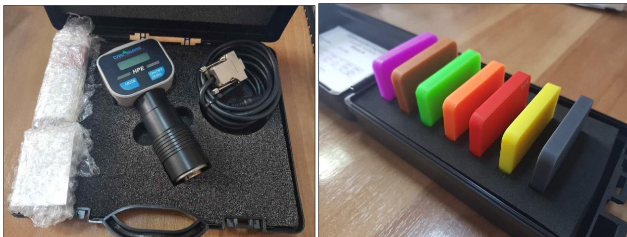
Figure 1. Shore A hardness tester and rubber test/calibration blocks
