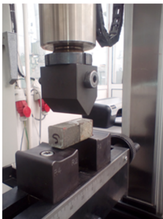
Fig. 1. Image of the samples used to determine the breaking strength by bending
