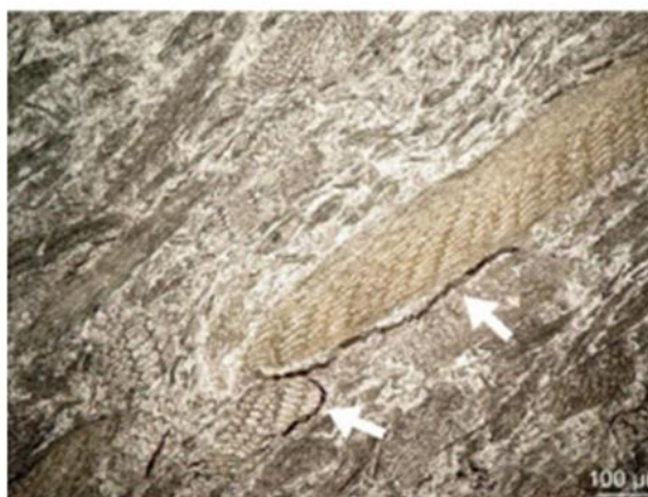
Figure 4. Microcracks localized on the contact between wood particles and plastic matrix [14]
