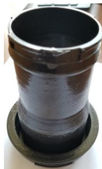
Fig. 7. Surface quality after vapor smoothing process
