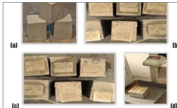
Figure 10. Concrete cube samples, their labelling and weighing [7,8]
