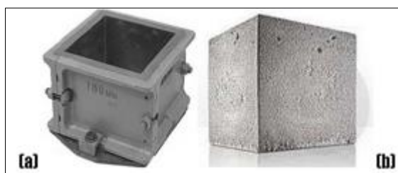
Figure 8. Preparing the samples [7,8] (a) 15 cm cube mould; (b) concrete cube sample
