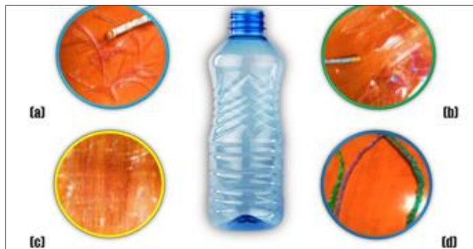
Figure 7. Preparing the PET reinforcements [7,8]: a) PET flat strips; b) PET chips c) PET mesh-shaped braids; d) PET rope strand
