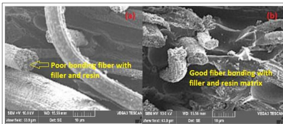
**Figure 5.** SEM image of (a) poor bonding (10% nano-silica) and (b) good bonding (20% nanosilica) for Coir fiber mats reinforced ER composites
