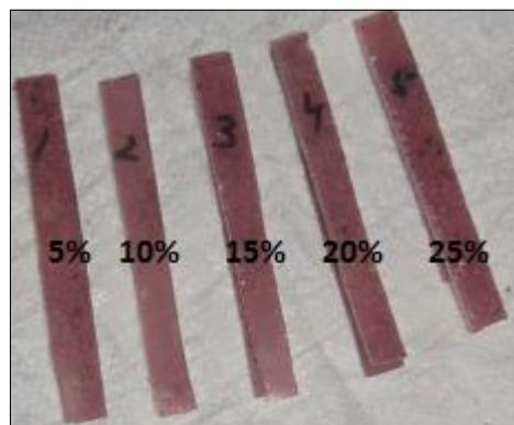
**Figure 3.** Flexural Specimen of Hybrid Composites
