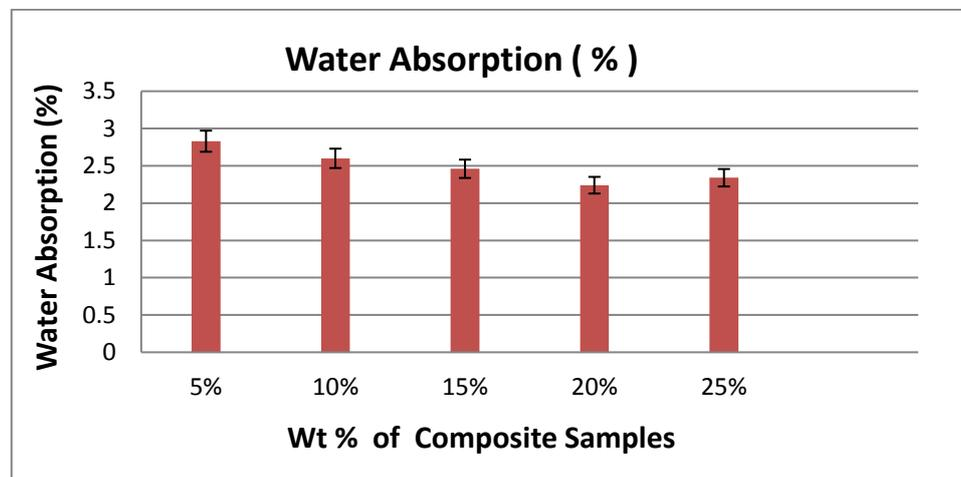
**Figure 9.** Water Absorption % for Hybrid Composites (Weight % of Nanosilica Particles (NP) reinforcement on Epoxy Resin (ER) / Coir Fiber Mats)
