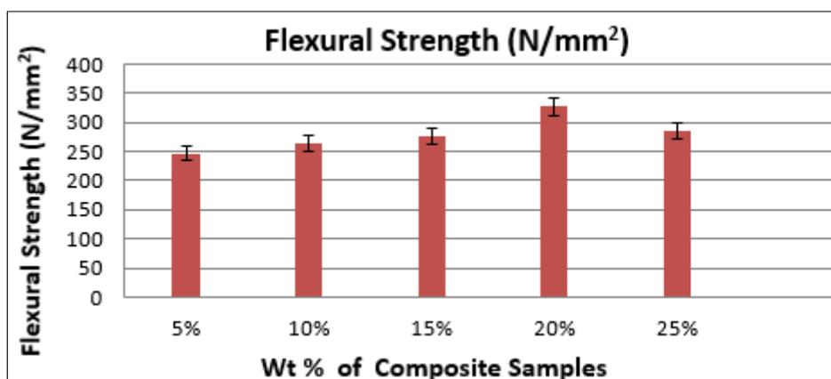
**Figure 6.** Flexural Strength results for Hybrid Composites (Weight % of Nanosilica Particles (NP) reinforcement on Epoxy Resin (ER) / Coir Fiber Mats)
