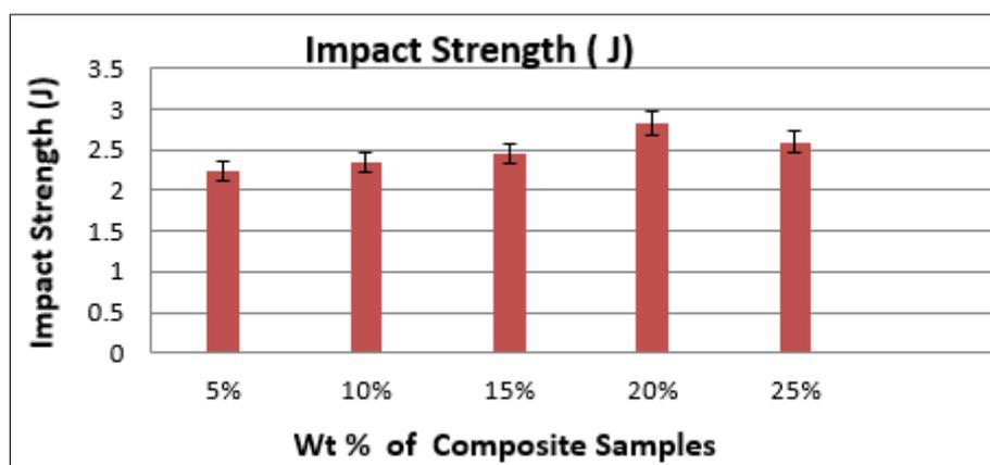
**Figure 7.** Impact Strength results for Hybrid Composites (Weight % of Nanosilica Particles (NP) reinforcement on Epoxy Resin (ER) / Coir Fiber Mats)
