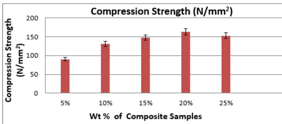
**Figure 4b.** Compression Strength results for Hybrid Composites (Weight % of Nanosilica Particles (NP) reinforcement on Epoxy Resin (ER) / Coir Fiber Mats)
