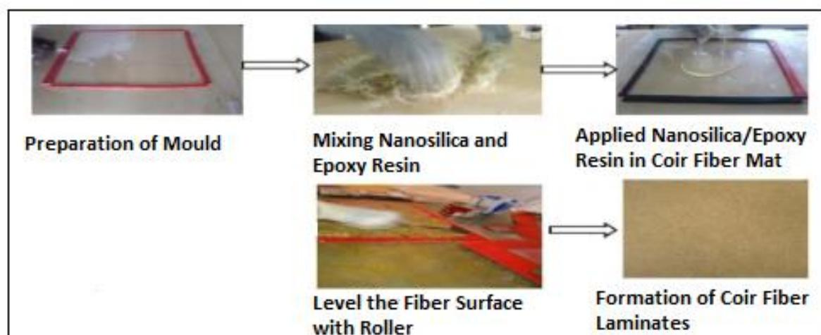
**Figure 1.** Hand layup technique for manufacturing of natural fiber mats (Coir fiber mats) reinforced epoxy resin blender nano-silica composite
