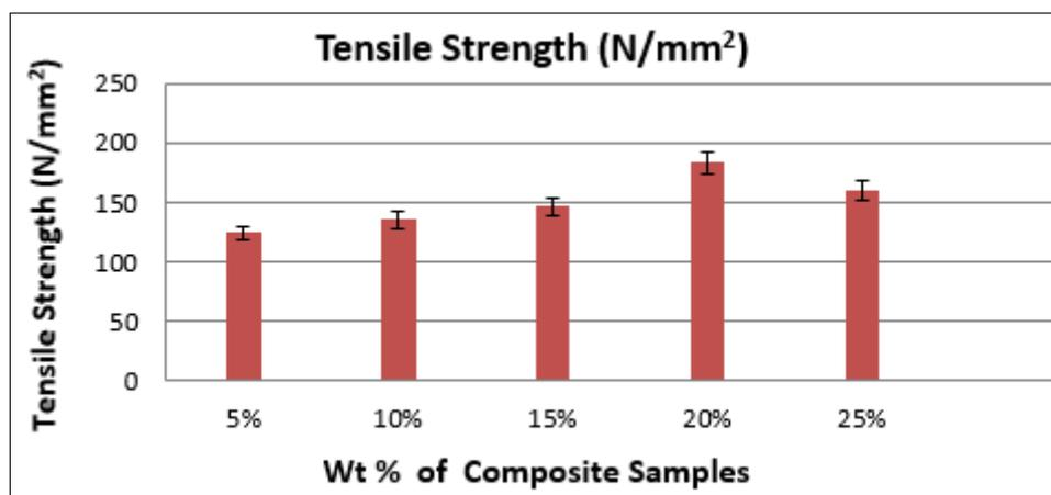
**Figure 4a.** Tensile Strength results for Hybrid Composites (Weight % of Nanosilica Particles (NP) reinforcement on Epoxy Resin (ER) / Coir Fiber Mats)
