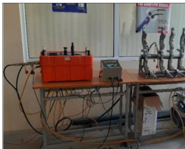
Figure 2. Work device for welding pipes
