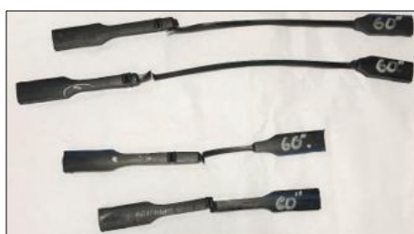
c. comparative aspect of some welded samples after the tensile test
