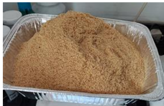
Figure 2. Wood dust, particle size <0.841mm
