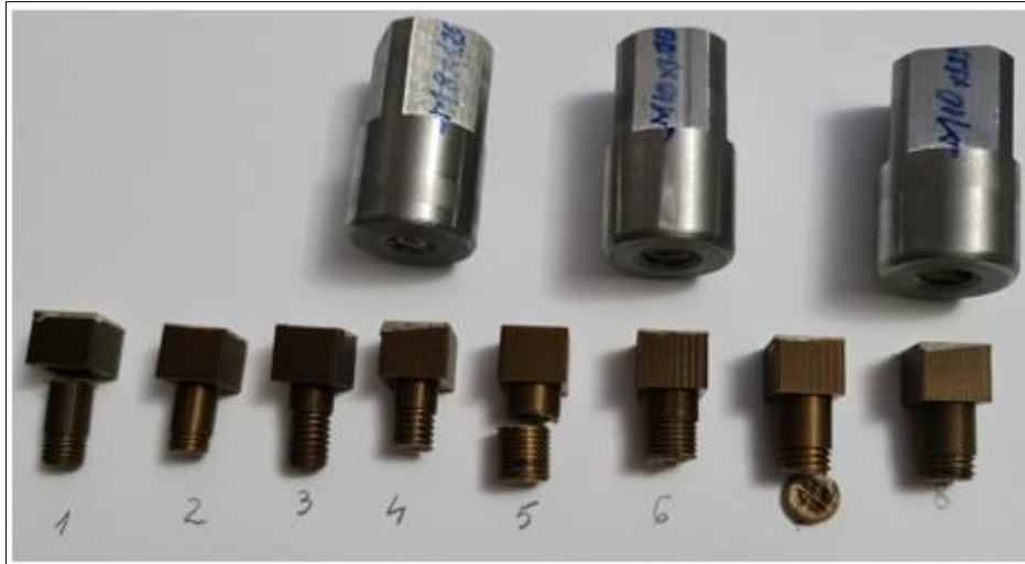
Figure 6. Test pieces (1-8) after performing the 8 experimental tests, revealing the initiation and possibly the development of the breaking process in different steps of the screws
