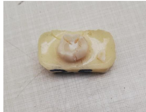
Fig. 7. Fracture line in a molar with nanohybrid restoration
