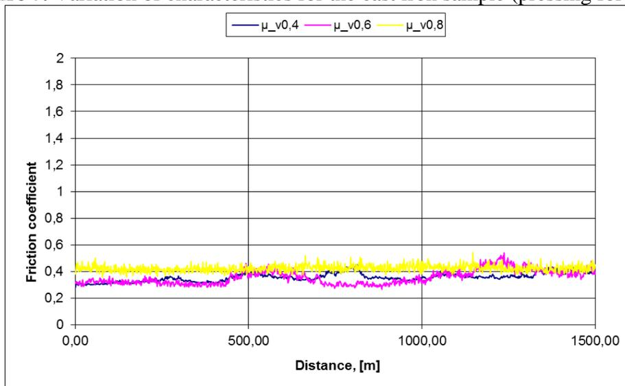
**Figure 8.** Variation of characteristics for the composite sample (pressing force  $F_2$ )
