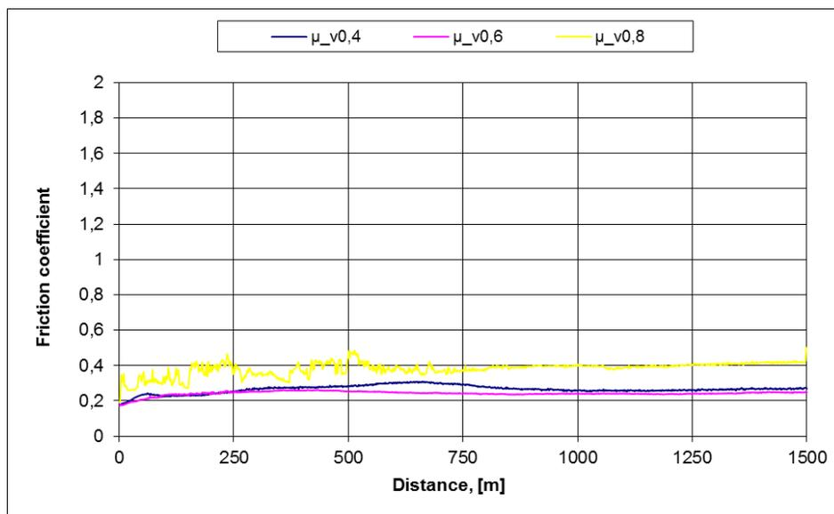
**Figure 9.** Variation of characteristics for the cast iron sample (pressing force  $F_2$ )
