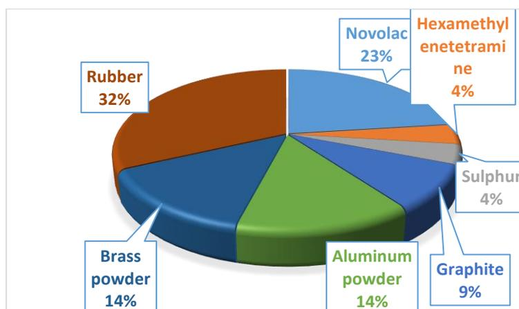
**Figure 2.** The recipe for the composite material sample
