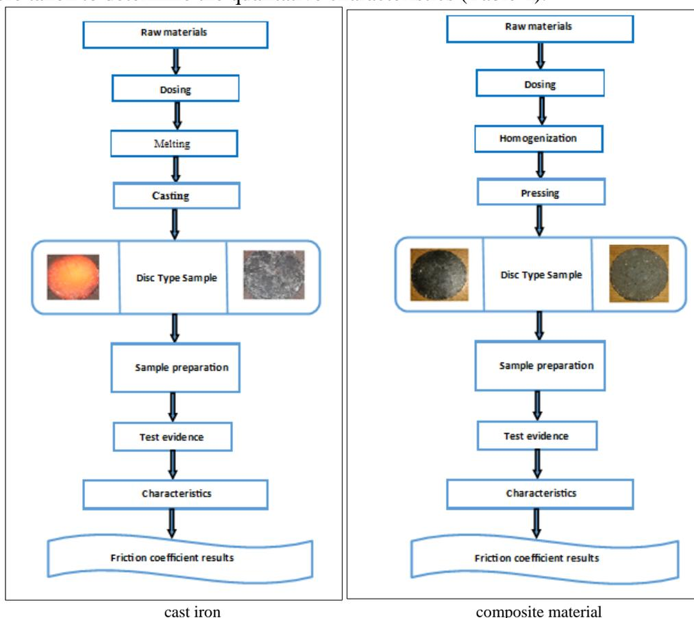
**Figure 1.** The technology of obtaining and testing the samples
