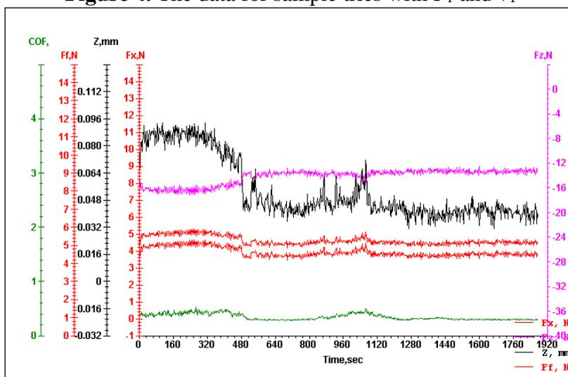
**Figure 5.** The charts of the measured parameters by the tribometer when testing the composite material disc sample, with  $F_2$  and  $v_3$
