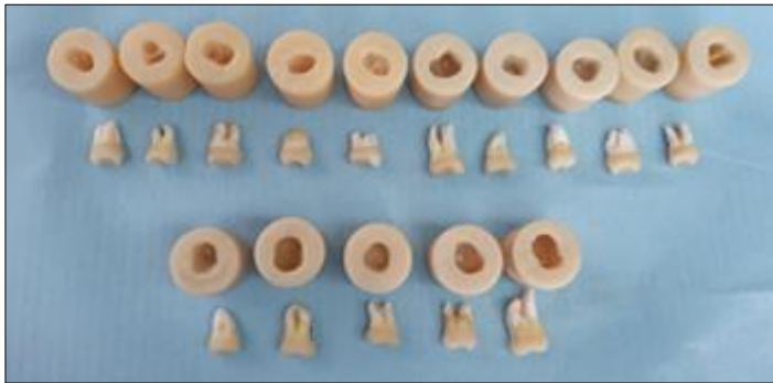
Figure 3. Selected tooth prepared for the experiment (roots were then coated with polyvinylsiloxane)
