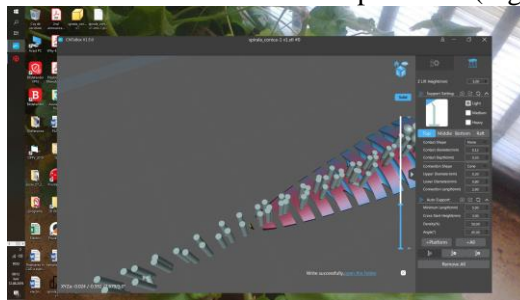
Fig. 14. Position of support for DLP printing red colour
