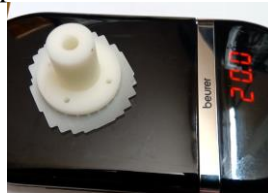
Fig. 19. Vertical printed position for threaded component
