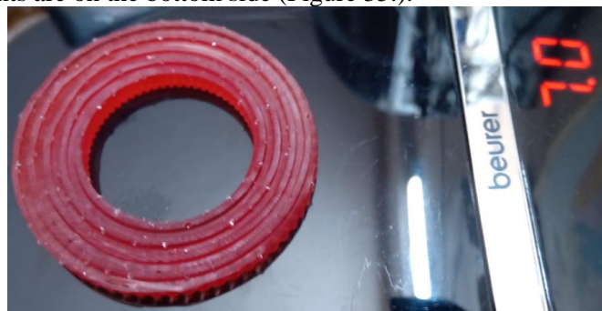
Fig. 34. 3D printed plan spiral with spiral bottom
