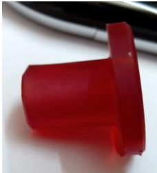
Fig. 24. Horizontal printed position for threaded component
