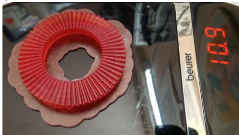
Fig. 29. 3D printed plan spiral with supports
